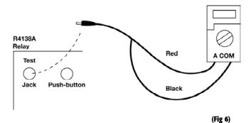
6. Insert cable connector plug into flame current test jack to put meter in series with flame lead (Fig 6). To stabilize meter reading, hold relay 2K in with one hand, press test push-button with other hand, read μA scale and release button. When normal pulsing is reestablished, release relay 2K. A stable reading, with the push-button depressed and 2K held in, of 4 to 4-1/2 minroamps is the minimum acceptable flame current.
