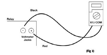
Meter connections for checking performance of lead sulfide photocell with R478B or R4074B relay.
